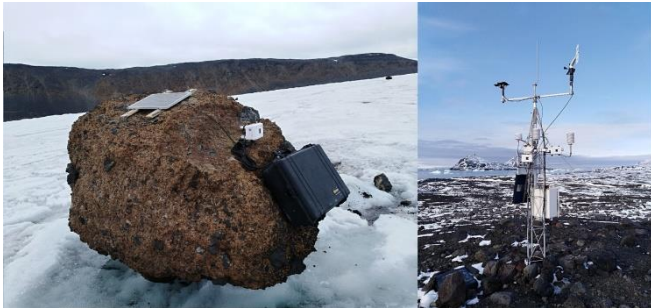
Fig. 4. Installed devices in EMBD, Vega Island to measure temperature and humidity (right panel) next to installed device on a rock in GBD to monitor glacier displacement (left panel).
