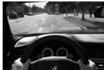
Fig.1: AR Example: a windshield with the path and driving information superimposed to the road
