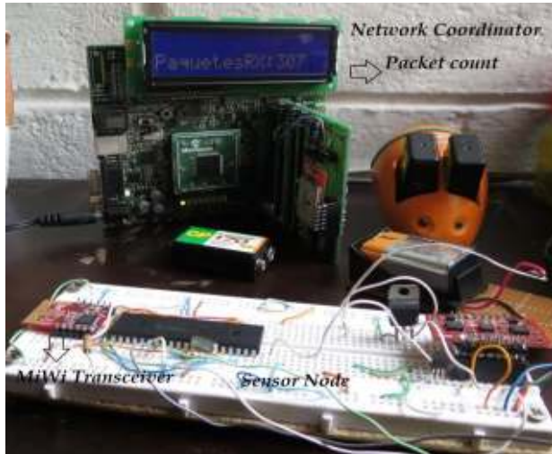
Fig. 9. Sensor node and the mains-powered specially developed PAN coordinator to conduct continuous operation tests.
