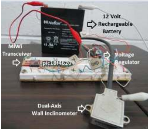
Fig. 11. Basic sensor node element arrangement to operate on the field.
