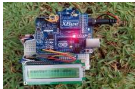
Figure 1 - Measurer prototype using Arduino Platform
