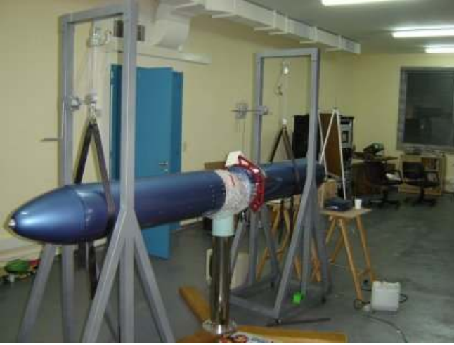
Fig. 1. SESCO - air-bearing testbed system
