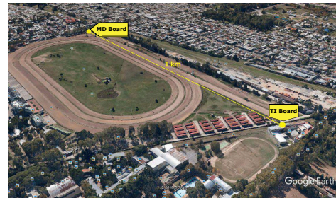
Fig. 4. 1 km link test developed in the hippodrome of La Plata city between the DM board and one of the TI evaluation boards (capture of Google Earth).
