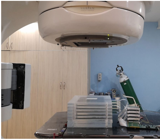
Figure 11 - linac and the acquisition system setup.
